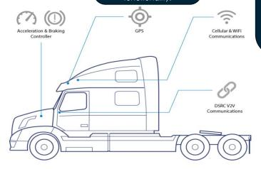
Cellular and Wifi modems connect vehicles through an encrypted channel to Peloton's cloud-based Network Operations Center (NOC). NOC tells trucks where and when they can platoon and under what conditions. Peloton minimizes cost of transmission by only sending high-priority data over cellular. Low priority is retained on truck until it reaches a WiFi hotspot.
