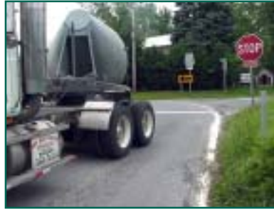
Truck encroachment into eastbound MD 407.
