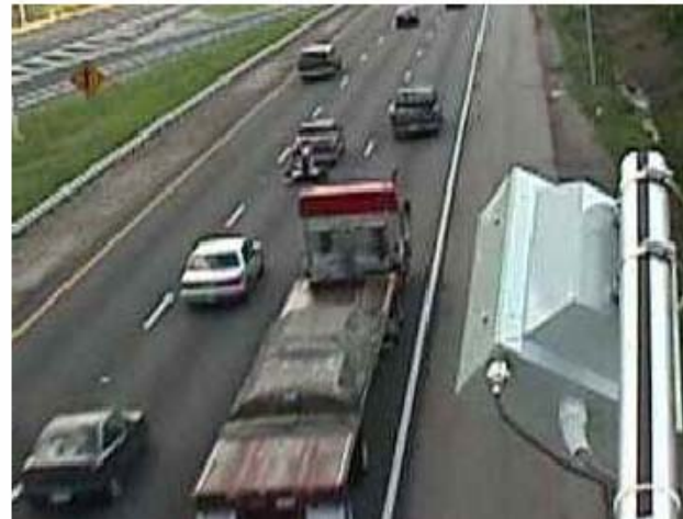
SmartSonic acoustic sensor. (Photograph courtesy of IRD, Saskatoon, SK)
