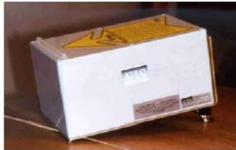
RTMS multizone presence-detecting microwave radar. (Photograph courtesy of Lawrence A. Klein).
