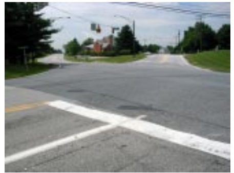
(Above) Sidewalks are missing on all approaches to the school. Traffic speeds are high, and turning movements are complex. Children cannot see the signals, and pedestrian signals are missing. This intersection may model well for a roundabout. Sidewalks are needed to area housing and other destinations.
